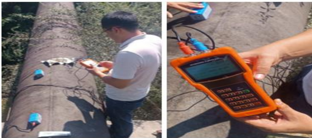
1-rasm. “Series CAM-3000H” markali ultra tovushli sarf o‘lchash qurilmasi orqali tadqiqot olib borish jarayoni.
